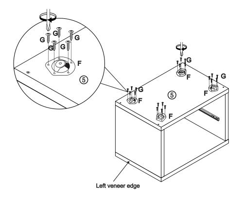
STEP 6: Fix legs  $\P$  to the metal plates  $\P$  .
