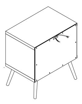
STEP 2: Fix bracket onto the wall using screws M4\*30MM. Join wallboard and the furniture with plastic sting.
