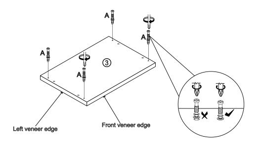
STEP 3: Attach top panel ③ to left side panel ① and right side panel ② with the cam locks ⑧ .
