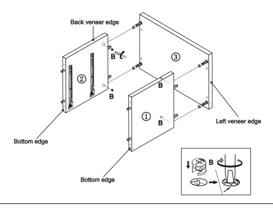
STEP 4: Attach bottom panel ® onto existing unit with screws ® .
